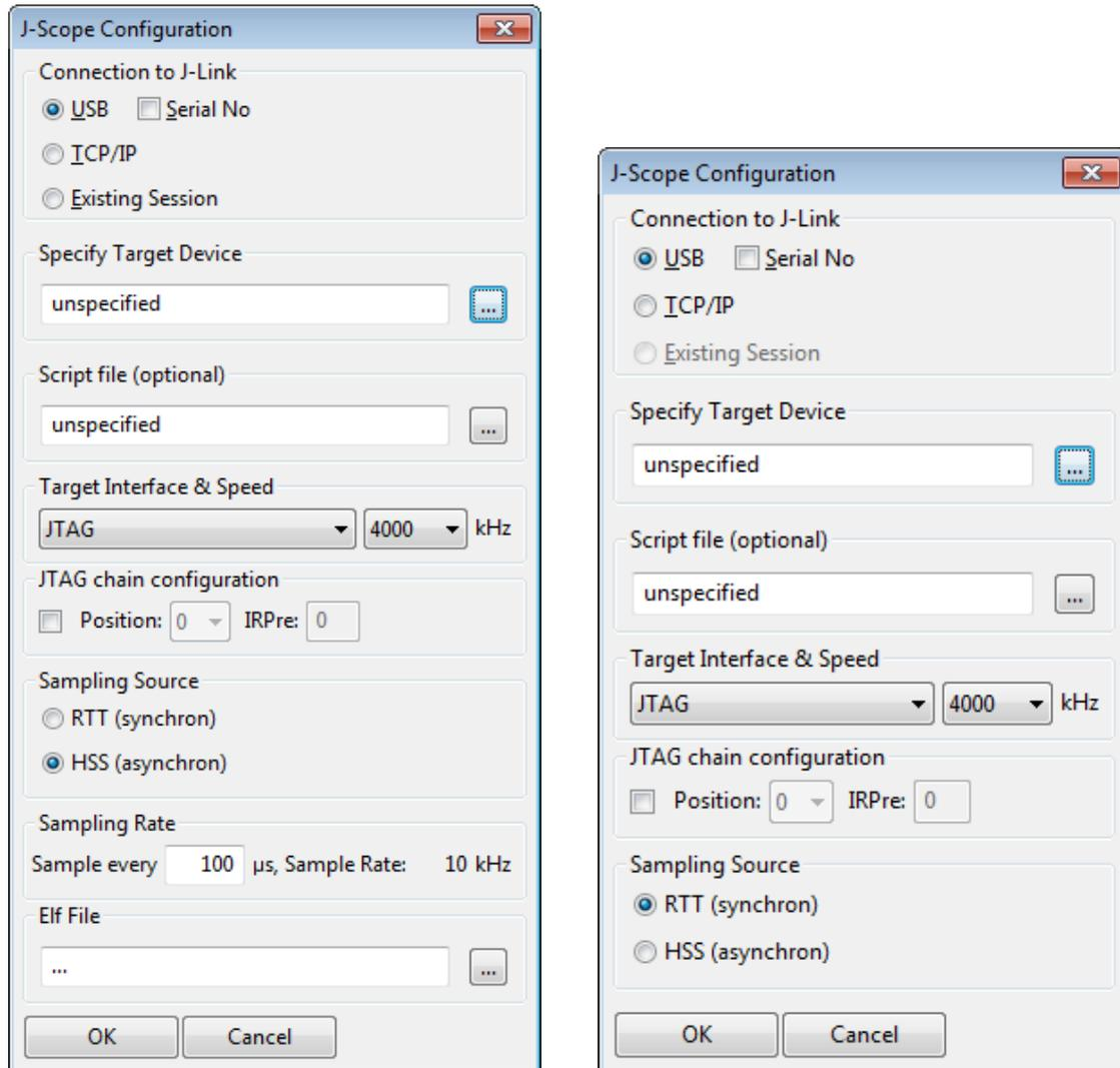
If J-Scope is used in standalone mode, using a dedicated connection to J-Link, choose “USB” or “TCP/IP” as connection type and optionally enter the serial number or the IP address of the J-Link to connect to a specific J-Link.
