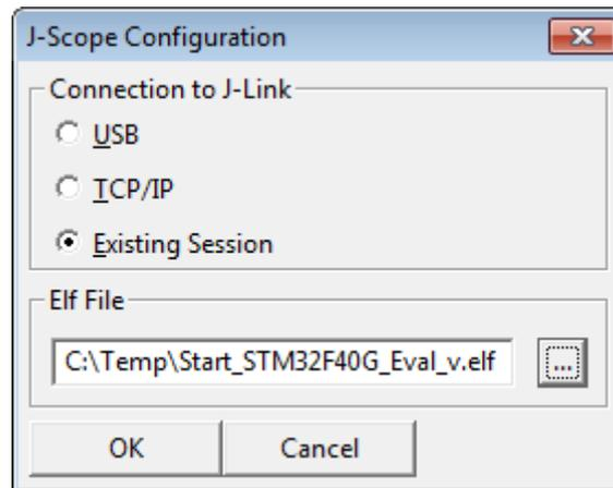
J-Scope can be used alongside other applications, e.g. a debugger, which are connected to the J-Link and share the connection to the J-Link. If J-Scope is used in this mode, select "Existing Session" as connection type. All target options will be disabled, as they are already determined by the running session.
